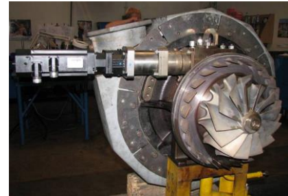
T/C with variable turbine nozzle vanes
