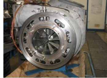
T/C with variable compressor inlet guide vanes
